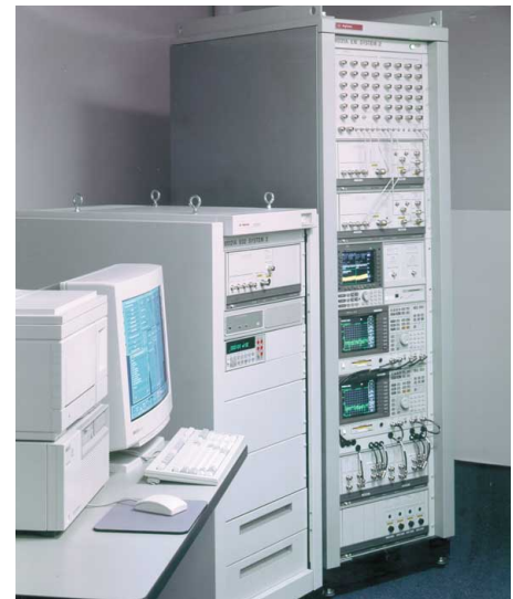
This Agilent satellite payload test system includes a switch matrix to route stimulus and response signals to 20 uplink and 20 downlink ports.
